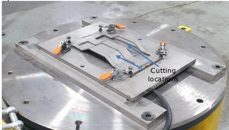
Figure 6 Laser cutting process demonstrated on GEL aerospace case study – laser processing (a) and resulting cut component (b).
