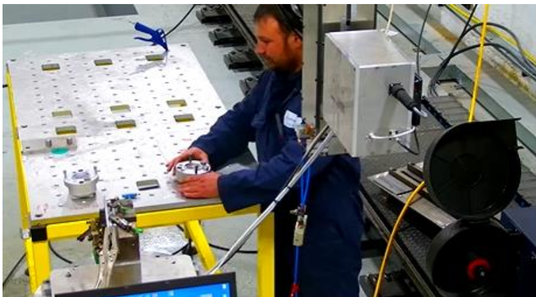
Figure 3 Operator at GEL laser cell, handling ModuLase end-effectors.
